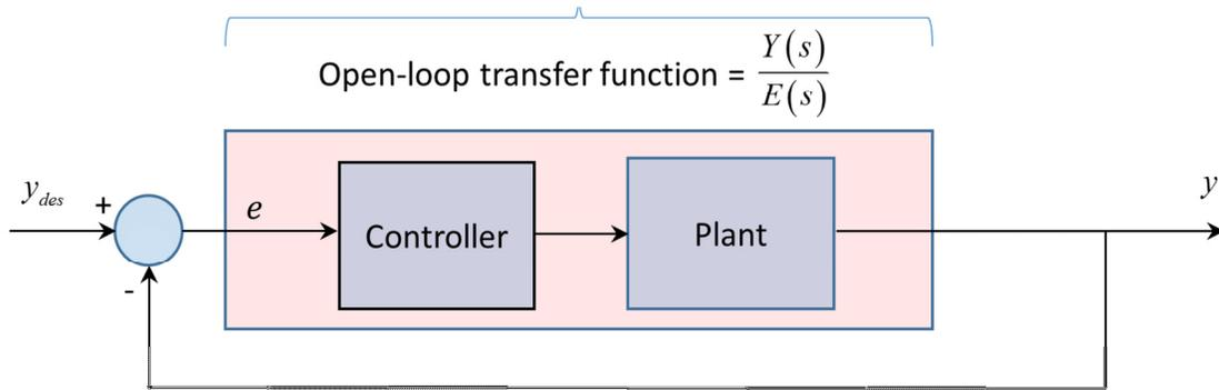
**Figure 6:** Open loop transfer function definition.
