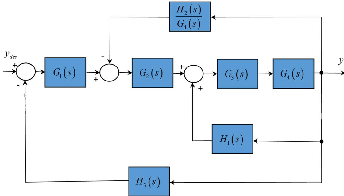
**Figure 7:** Block diagram of a process with three sensor feedback.
